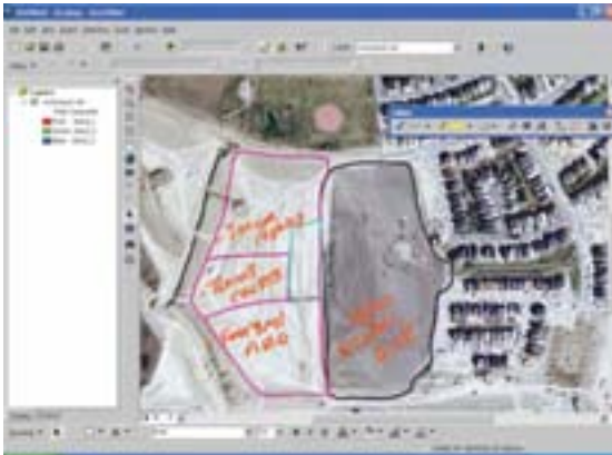
Sketches and notes created in ArcMap on the Tablet PC are geographically referenced and can be saved as map graphics or as annotation features in the geodatabase.
