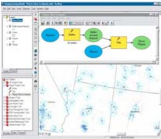
ArcToolbox and ModelBuilder are the cornerstones of the ArcGIS geoprocessing framework used for automating tasks and for spatial analysis.
