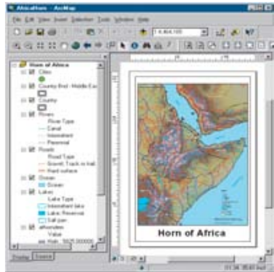
The main application in ArcGIS is ArcMap, which is used for all mapping and editing tasks as well as for map-based query and analysis.
