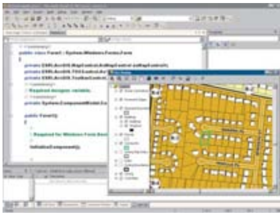
An example of a custom ArcGIS Engine application being developed with VB. A map control, a table of contents control, a menu, and a toolbar have been added to this VB form. The map control is associated with an ArcMap document (a .mxd file) used to draw and query interactive maps.
