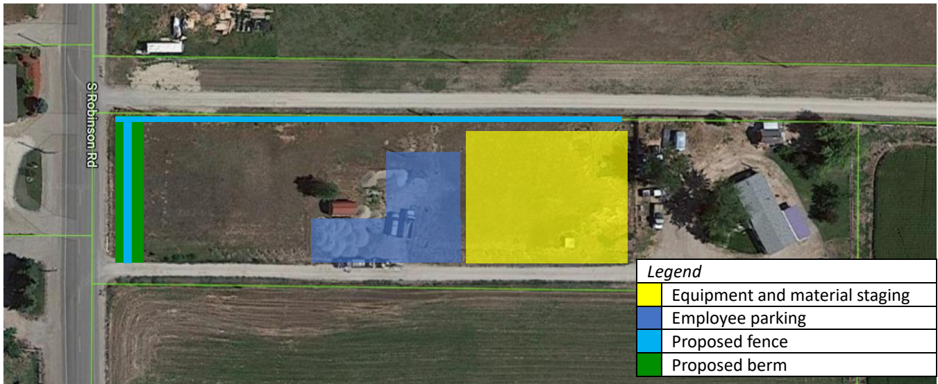
Image 2. Updated site plan with proposed changes to the staging area with the removal of dirt staging.
