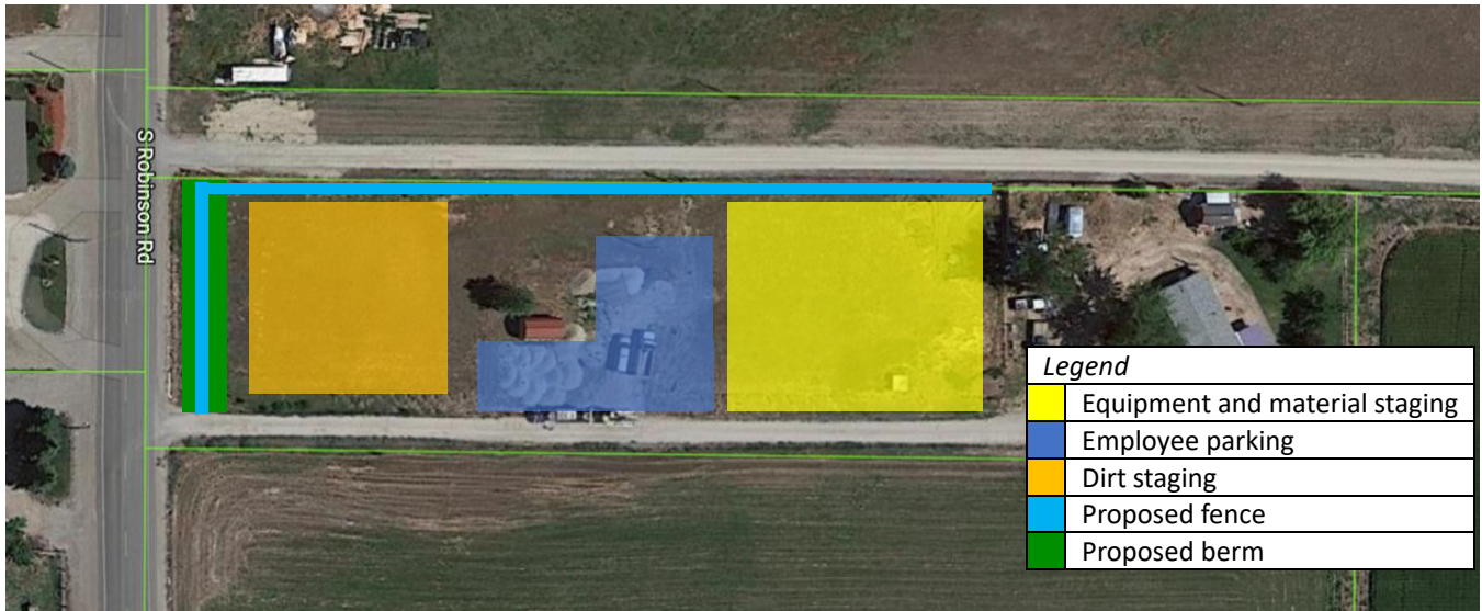
Image 1. The original site plan that went before the Planning and Zoning Commission with proposed fencing and berm.
