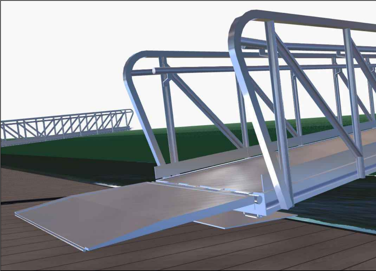
GANGWAY ROLLING CONNECTION TO DOCK WITH ROLLING DECK PLATE. PROVIDE BRACKET CONNECTION ON UPPER END
